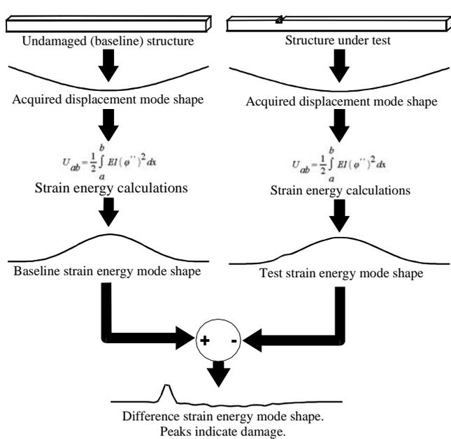
Fig. 3. Illustration of modal strain energy method.
