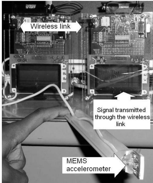
Fig. 4. A prototype of the WISAN nodes.
